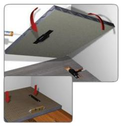
Apply a wavy line of acrylic sealant (e.g. Marmox Multibond or Jackoboard Board Fix, not supplied) across the edge of the shower tray base. Place the shower tray into position and bed down onto the adhesive cement. Check that the shower tray is level in both directions using a suitable level.
