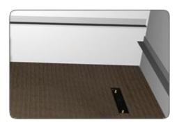
Paint acrylic primer onto the edges of the shower tray and onto adjoining walls, covering at least 50mm of tray and wall. Allow to dry. From a roll of sealing tape cut to suit the width of the shower tray and the length of the shower tray. Temporarily place a waterproofing internal corner into position and mark around it with a pencil. Once marked it can be removed. This is to show where you need to apply Tanking Solution. Repeat for any other corners.
