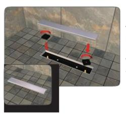
The linear drain is supplied with 2 or 4 No. square black plastic height adjustment nuts. Screw these onto the protruding bolts pre-fitted within the linear drain and adjust to suit your thickness of tile and adhesive. The drain should aim to be fitted flush with the finish tile.
