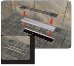
Various options are available to accessorise the linear drain including a tile able drain cover option to give a more bespoke finish to your shower room. These are installed in the same way as above; just adjust the black plastic height adjustment nuts to suit. Leave for at least 24 hours before using the shower.
