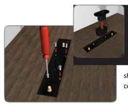
Line up the linear drain bowl with the drain top prefitted within the shower tray and connect the two together using the four bolts provided and a suitable cross headed screwdriver. Ease the shower drain internal bowl into place then ease in the drain top as shown applying a little gentle pressure so that it seats correctly.
